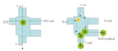
Similar physical gates and billiard balls could be constructed to replicate the OR and NOT gates. As you may recall from the prior blog, all Boolean logic operators can be created using combinations of these three gates, so a theoretical computer constructed entirely of wood and billiard balls, could replicate the results of any existing computer.
