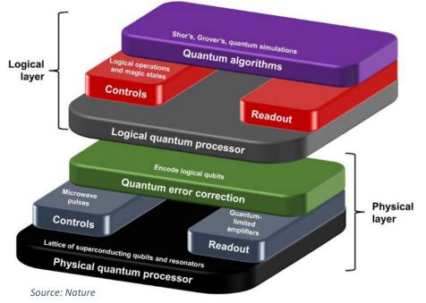
As this graphic shows, there are various aspects of the physical creation and manipulation of qubits (the bottom section of the graphic) along with software needed to control the logical layer. Also, covered in a prior post, there are various ways to create qubits, often requiring cryogenic temperatures and/or detailed laser or radio frequency controls.
