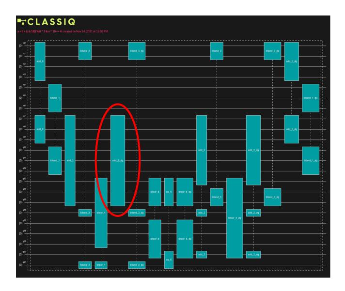
You can see the various qubits listed along the y-axis and the various functional blocks that comprise the algorithm. If users want to drill-down to see what is within a given block (such as the block above circled in red), they simply click the "+" sign and it is further broken out visually as shown below:
